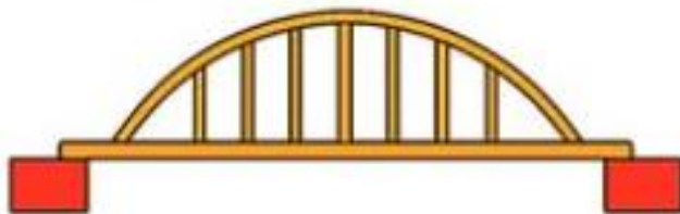
TIED ARCH BRIDGE
